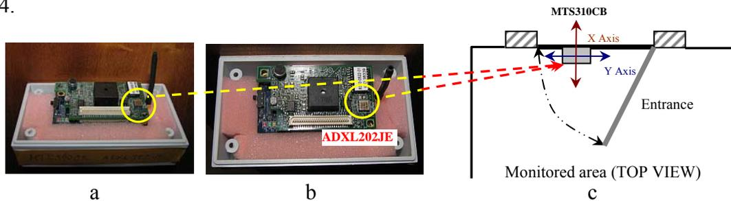
Figure 4 Simplified test bed for ADXL202JE
