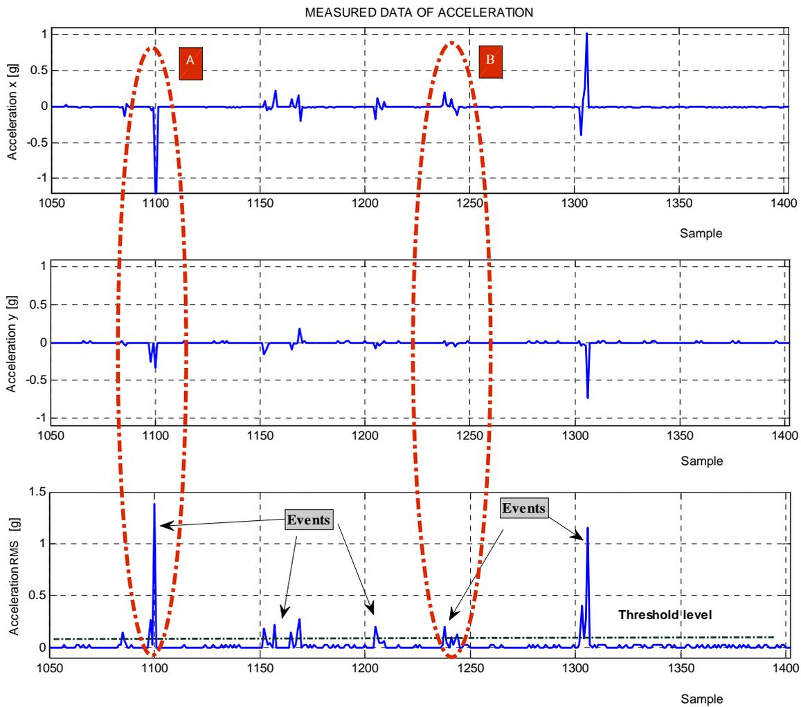
Figure 5 Waveforms of the measured acceleration data during a violation of monitored area
