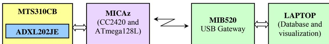
Figure 1 The basic arrangement of experimental measurement system
