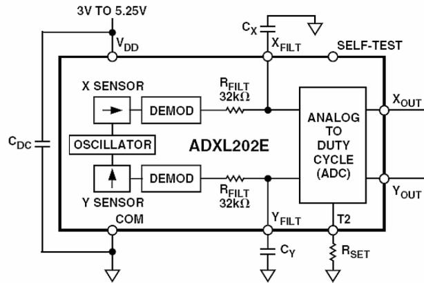
Figure 3 Block diagram of the ADXL202JE
